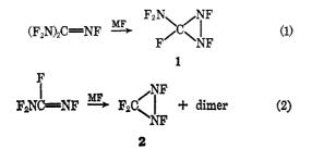
The reactions were usually carried out by condensing either pentafluoroguanidine or tetrafluoroformamidine into an evacuated Pyrex glass reactor containing the alkali metal fluoride. The reactor was then allowed to warm to room temperature. Both liquid-solid and gas-solid reactions could have occurred under these conditions. After the desired time at room temperature, the products were separated by fractionation in a vacuum line and/or fractional codistillation.<sup>5</sup>
